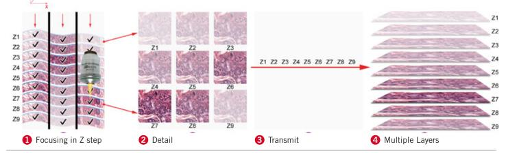
Z-Stack - Used for slide with 3D reconstruction
